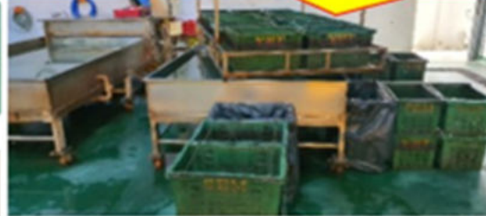
Tank 1 : water mixing with Chlorine (Cl)
